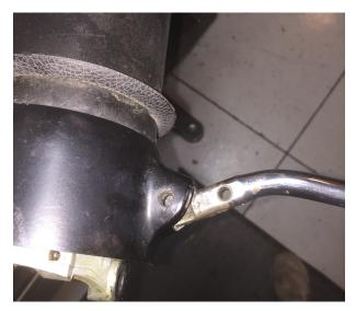
Install the shift lever at such an angle so the tip does not dislodge the spring, but slides above the spring tip and deep into the space for the tip to engage the detent plate.
