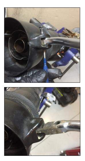
1. Remove the original shift lever by simply pushing the pivot pin out of the bowl. A small punch or similar tool may be used. Gently tap it upward with a hammer and the pin will come up and out.
