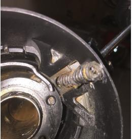
3. With a small flat blade screwdriver, firmly pry the spring out of the seat and towards the driver. If will fall out into the shift bowl and/or onto the floor (maybe not now, but ultimately it will drop out)
