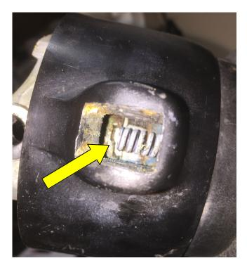
7. Look into the hole and determine the spacing between the new shift return spring and the opening available to insert the shift lever. It should look like this.
