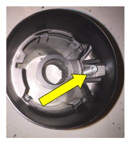
We have illustrated a top view of the shift bowl in the "Neutral" position to show you where and how the spring seats into the bowl.
