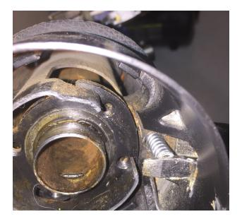
6. Once you feel the spring is partially seated in the bowl, using a flat blade screwdriver, firmly pry the spring FARTHER into the seat. Once fully seated, it should be fairly tight in position.
