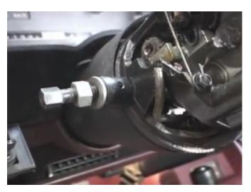
2) With the nut threaded most of the way onto the puller shaft, thread the small threaded end of the puller shaft into the pivot pin by hand.
