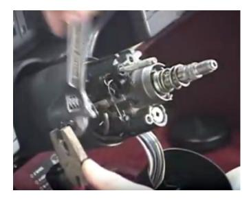
5) Using an open end wrench, crescent wrench or ratchet and socket, continue to tighten the nut on the puller shaft. This should draw the pin out of the housing smoothly.
