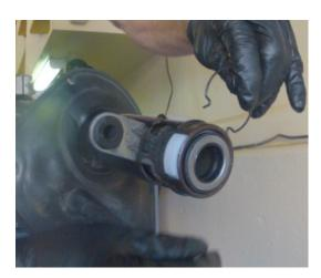
Grease the inside of the bearing for the shaft to slide more easily during assembly.
