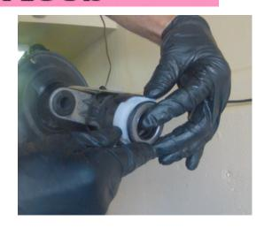
3) Centering the bearing (it floats slightly) carefully tap the retaining ring over the tube aligning the slots and opening with the housing slots and openings.
