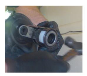
4) Install the snap ring into the three grooves. Make sure the snap ring seats in all three openings. You may need to tap it into position.
