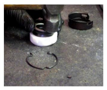
1) Insert the bearing into the bearing housing using either pressure from the palm of your hand or a gentle tap hammer. The smaller edge of the bearing will snap into place into the larger opening of the housing.
