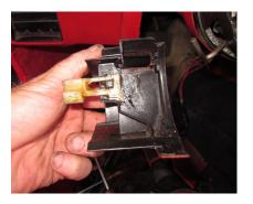
place the dimmer actuator inside the dimmer cap as shown. The grease will keep it in place.
