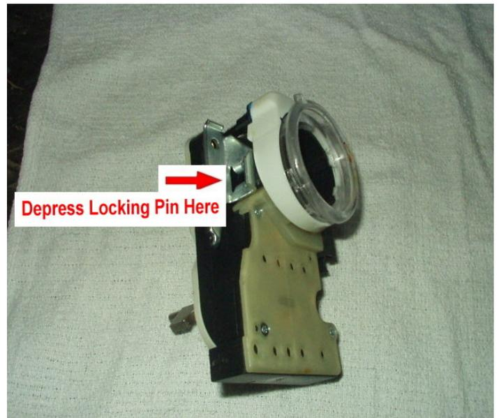
Once depressed, the lock cylinder will slide out of the switch.
