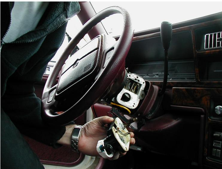
Lower the switch assembly to remove the wire connectors.
