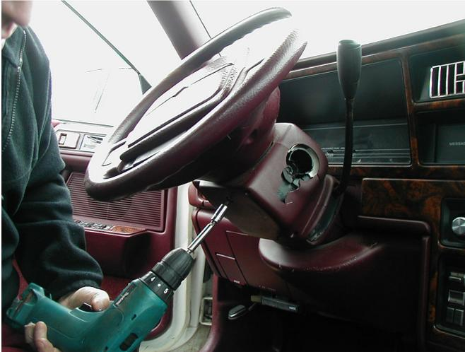
2) Remove the lower steering column cover. This design uses 2 screws to hold the covers together and a 3rd holding the lower cover to the column.
