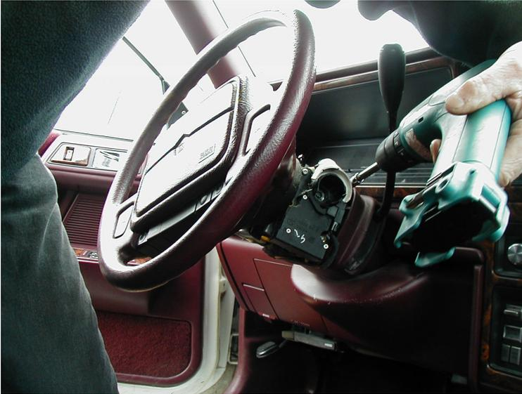
Remove the ignition switch assembly with (or without) the lock cylinder. These 3 bolts are also 20 torx, but are tamperproof, requiring a different socket.
