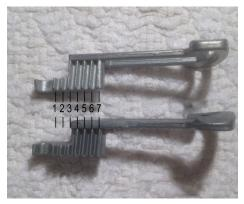
Although both gears have 7 teeth, they are distinctly different at the other end---where they connect to the rod that runs down the column.
