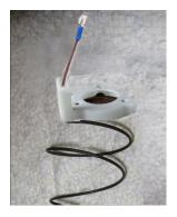
Attach a spade connector to the exposed end of the wire (or whatever connector you need to attach to the horn pad) and reinstall the steering wheel with the spring touching the horn contacts in the column.
