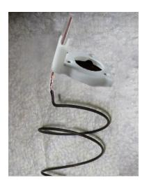
Reinstall the spring into the broken plastic stem with the wire going through the stem and steering wheel. (All completed with the steering wheel just flipped over)
