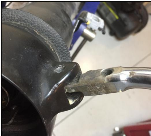
2. Pull the shift lever away and out of the column.
