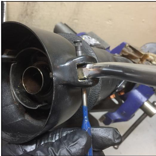
1. Remove the original shift lever by simply pushing the pivot pin out of the bowl. A small punch or similar tool may be used. Gently tap it upward with a hammer and the pin will come up and out.
