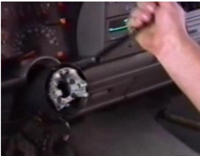
11. Check the shifter and the lever return tension by shifting to all the shift positions.
