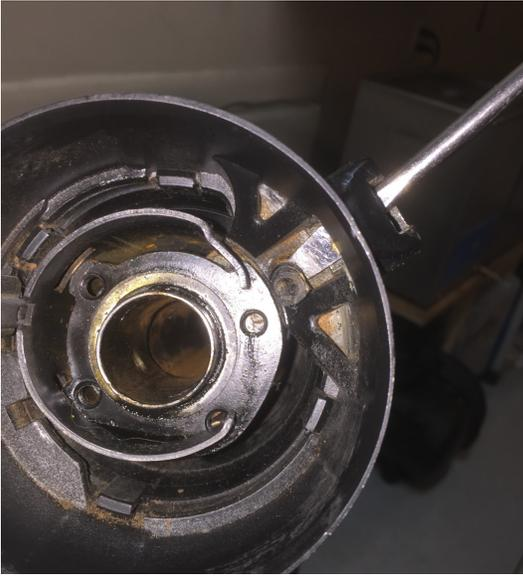
3. With a small flat blade screwdriver, firmly pry the spring out of the seat and towards the driver. If will fall out into the shift bowl and/or onto the floor (maybe not now, but ultimately it will drop out)
