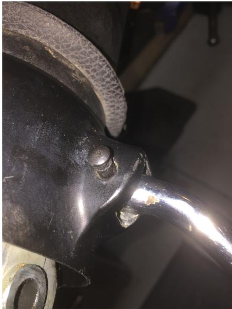
9. Once fully inserted, align the holes for the pin by compressing the shift spring with the lever (towards the dash)
