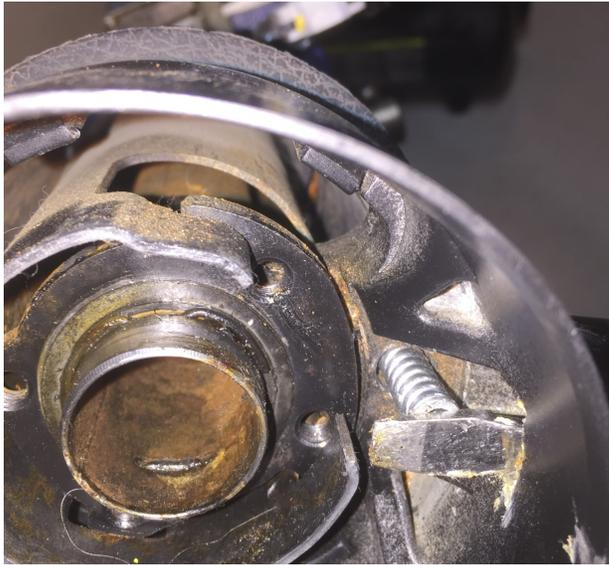
6. Once you feel the spring is partially seated in the bowl, using a flat blade screwdriver, firmly pry the spring **FARTHER** into the seat. Once fully seated, it should be fairly tight in position.
