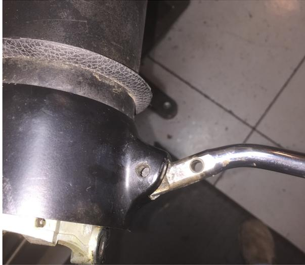
8. Install the shift lever at such an angle so the tip does not dislodge the spring, but slides above the spring tip and deep into the space for the tip to engage the detent plate.
