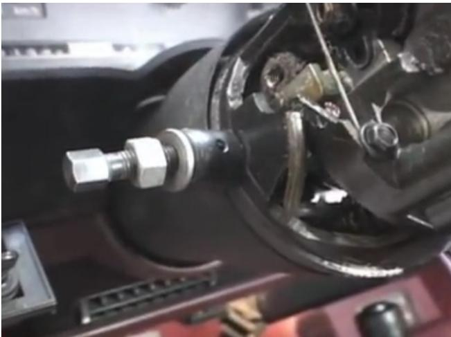
2) With the nut threaded most of the way onto the puller shaft, thread the small threaded end of the puller shaft into the pivot pin by hand.
