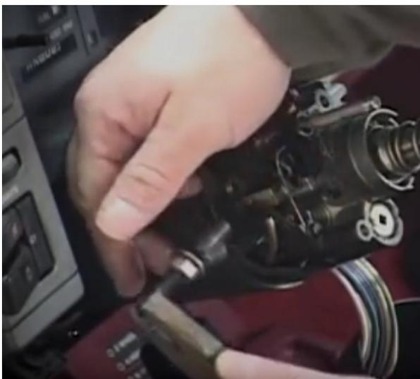
7) Once you fully tighten the nut on the shaft, the pin should come out easily. The last few threads can be done by hand.
