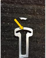
The first step is to cut open the inside area using a hack saw blade. Cut it at a 45° angle to open as much area as possible.
