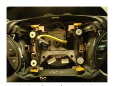
4. Remove the center bolt and remove the steering wheel. You may be able to remove it by wiggling it side to side (**PUT THE BOLT BACK IN FIRST**), otherwise, use a steering wheel puller
