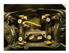
4. Remove the center bolt and remove the steering wheel. You may be able to remove it by wiggling it side to side (**PUT THE BOLT BACK IN FIRST**), otherwise, use a steering wheel puller
