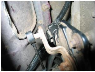
15. Remove shift cable from steering column lower mounting bracket by pushing tab on cable in and sliding cable off bracket.
