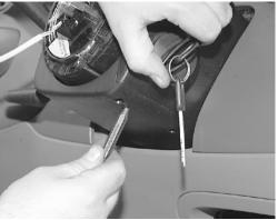
9. Remove three (or four) screws from lower steering column shroud and remove both shrouds from column.
