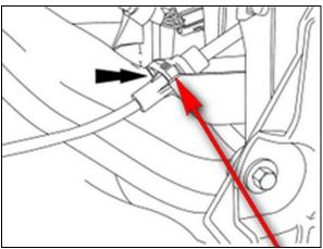
16. Disconnect ignition switch by loosening bolt and removing connector. The bolt is part of connector and will not come out of the connector.
