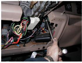
18. Remove steering column from vehicle.
