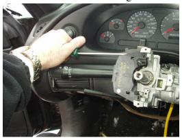
13. Remove pinch bolt from steering shaft coupling at the bottom of the column. Slide lower coupler off the end of the steering column.
