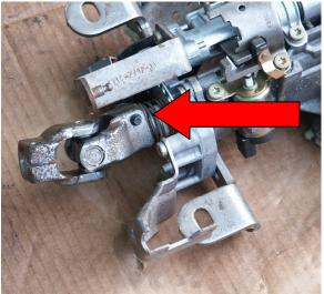
14. Disconnect shift cable from shift lever pivot at the bottom of the column (above the column)
