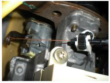
12. Remove two 20 torx screws and two electrical connectors from multifunction switch. Remove multifunction switch from steering column.
