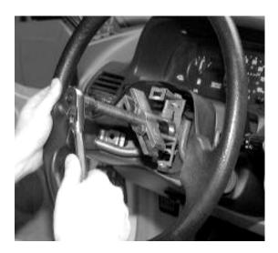
6. Remove steering column tilt release lever by unscrewing it
