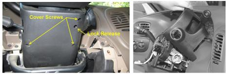
9. Remove instrument panel reinforcement brace if so equipped).
