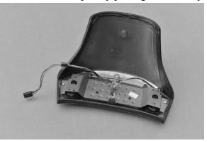
3. Remove the center bolt and remove the steering wheel. You may be able to remove it by wiggling it side to side (**PUT THE BOLT BACK IN FIRST**), otherwise, use a steering wheel puller
