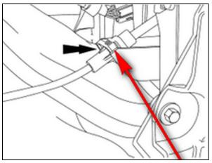
15. Disconnect ignition switch by loosening bolt and removing connector. The bolt is part of connector and will not come out of the connector.
