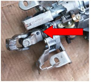
13. Disconnect shift cable from shift lever pivot at the bottom of the column (above the column)
