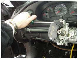
12. Remove pinch bolt from steering shaft coupling at the bottom of the column. Slide lower coupler off the end of the steering column.
