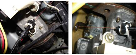
11. Remove two 20 torx screws and two electrical connectors from multifunction switch. Remove multifunction switch from steering column.
