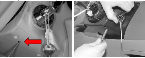
8. Remove three (or four) screws from lower steering column shroud and remove both shrouds from column.
