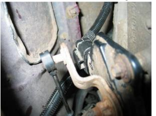
14. Remove shift cable from steering column lower mounting bracket by pushing tab on cable in and sliding cable off bracket.
