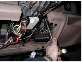
17. Remove steering column from vehicle.
